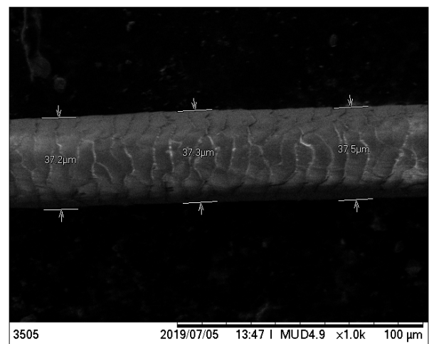
Figure 5: SEM image of a strand of hair using a Hitachi TM3030Plus Scanning Electron Microscope.
